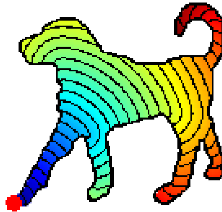
Geodesic distances from Fast Marching Algorithm
